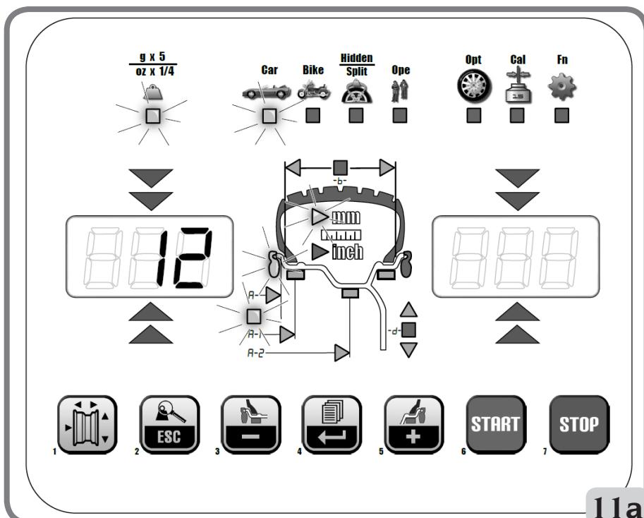
When the measurement is stored, the value of the distance acquired by the machine will remain visible on the left display:
