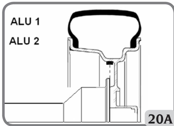
Some minor residual unbalance may remain at the end of the spin test due to the considerable difference in shape found in rims with the same nominal diameters. Therefore change the value and position of the previously applied weights based on the configuration performed in the programme "SELECTION OF ADHESIVE WEIGHTS APPLICATION POSITION" until an accurate balance is obtained.
