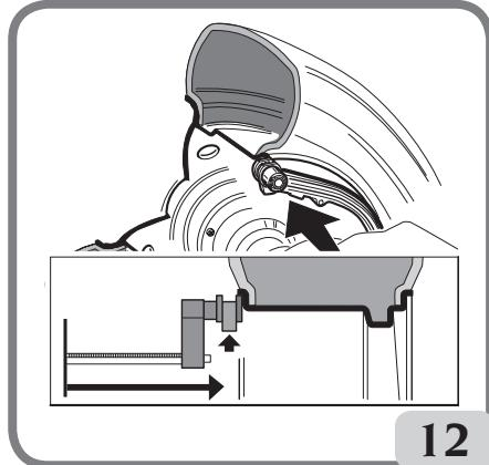
Take great care to position the arm correctly so as to ensure accurate data reading.
