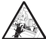
Never use the wheel spin shaft as a lifting point for the machine.
