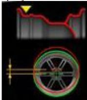
the radial run-out of the inner tyre bead (1<sup>st</sup> harmonic);
