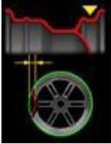
the radial run-out of the outer tyre bead (peak-peak);
