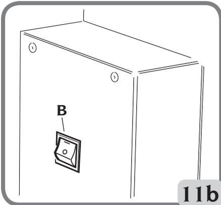
At start-up, the wheel balancer performs a series of control tests and displays the message “please wait”. If no anomaly is detected, it displays the customisation data and mark.
