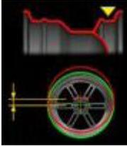
the radial run-out of the outer tyre bead (1<sup>st</sup> harmonic);
