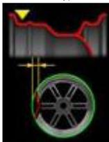
the radial run-out of the inner tyre bead (peak-peak);
