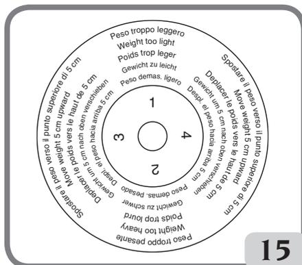
Bear in mind that a counterweight positioning error of just a few degrees may lead to a residual unbalance as large as 5-10 grams during the verification phase, especially in the case of large unbalances.
