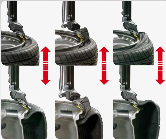
● **TOP BEAD DEMOUNTING PROCEDURE HEAD UNIT.** The demounting procedure uses the same working movements but absolutely no effort is required from the operator thanks to the “Leva la leva” technology incorporated in the mount/demount head (patented). The mounting procedure is exactly as before, and just as quick and convenient.
