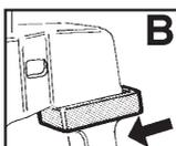
C- For the tool to be positioned correctly, the insert (3, Fig. 37) must be against the edge of the wheel where the vertical wall begins.
