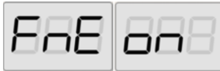
Fig. 28: Enabling imbalance display in high resolution
